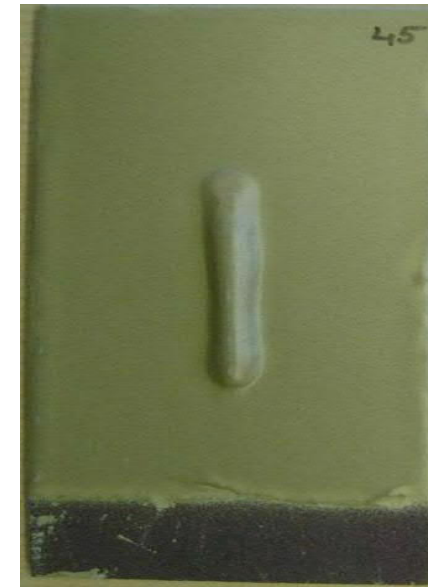
Alkylated amine epoxy 2 x 350 \mu m (14 mils)
