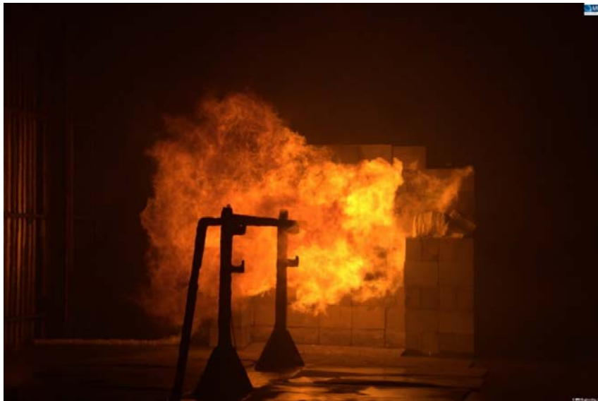
Figure 5 ISO22899-1 jet fire test
