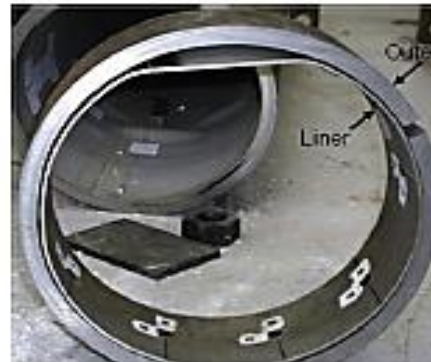
Lined pipe, (a) photo after experimental testing (Focke, 2007) and (b) wrinkled liner pipe (Hilberink, 2011).
