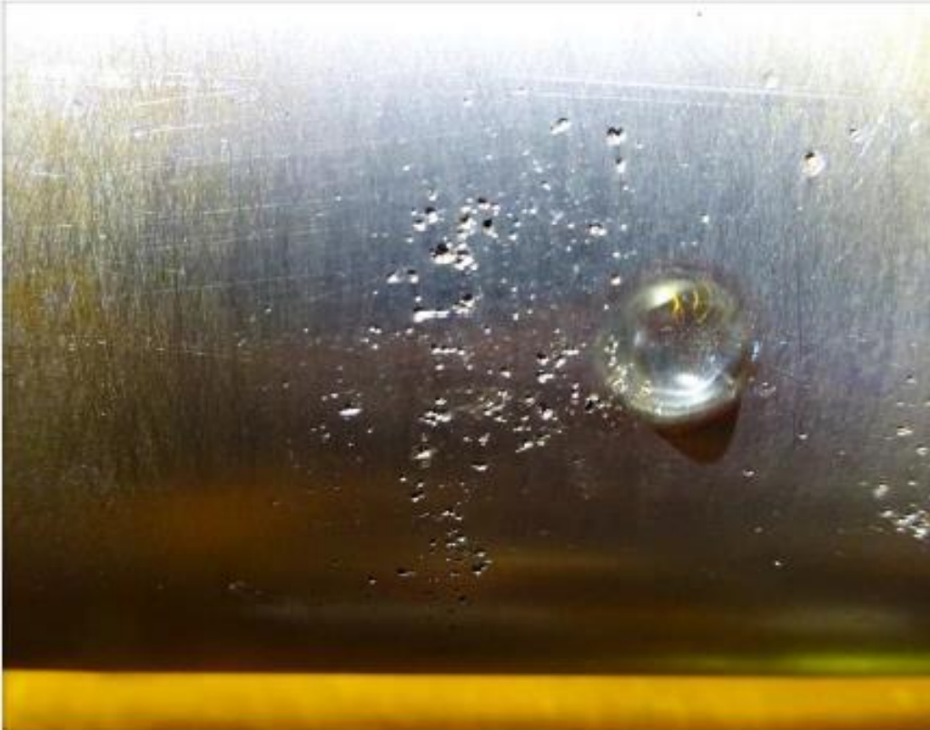
Poor Fabrication / Material Selection Practices – 316L Weeps + Pitting under ID Labels
