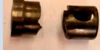
Stress Corr. Crack
