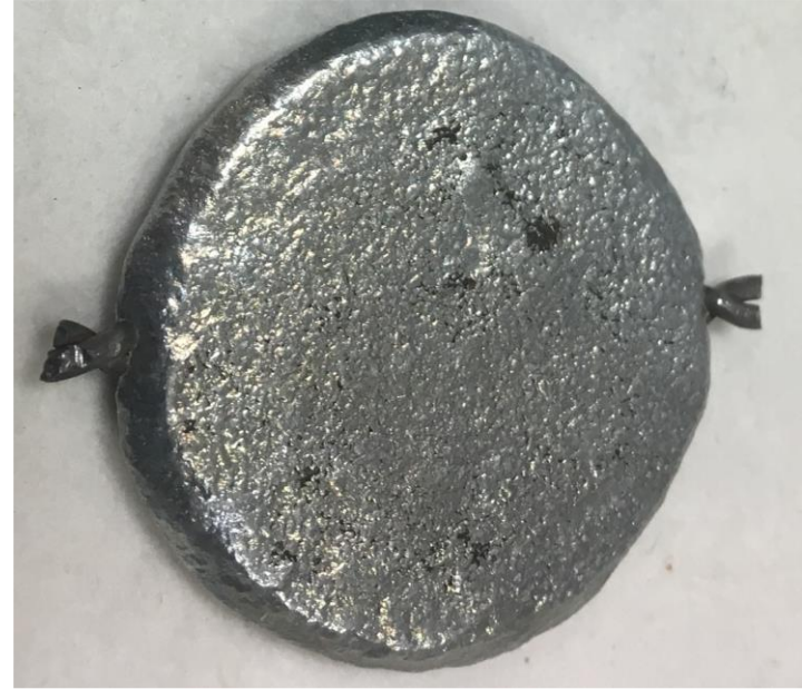
Anode after corrosion products removed
