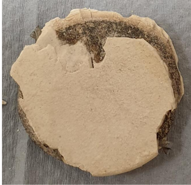
Condition of anode after 20 years
