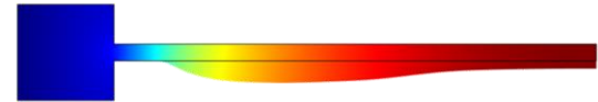
Top: Polarization curve taken from experimental data Bottom: Electrolyte potential and simulated geometry after 72 h
