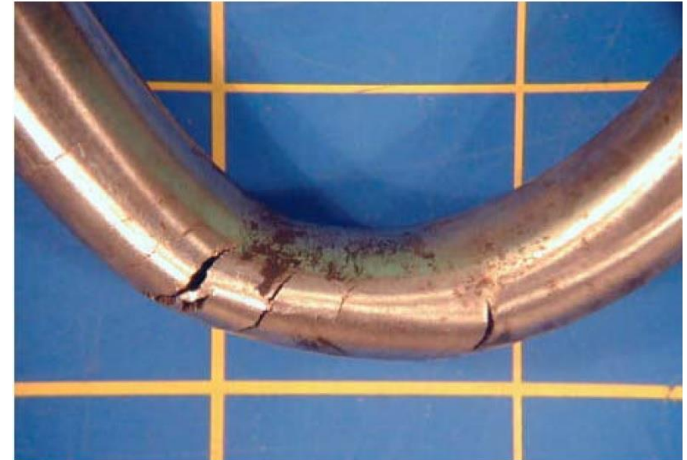
External cracking of Type 304SS instrument tubing under insulation (API 571)
