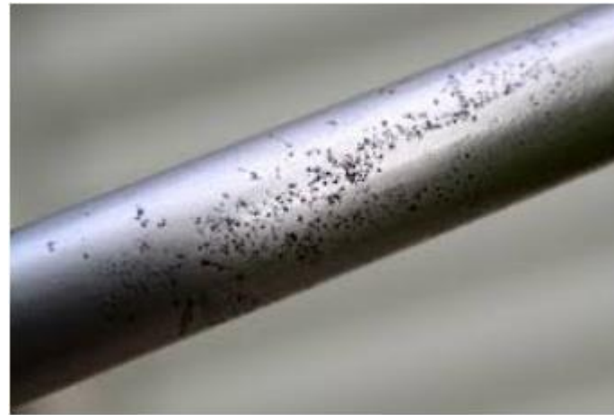
Stainless steel External Pitting Corrosion www.materialgrades.com
