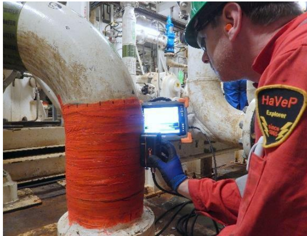
Inspections under non-conductive layers, e.g. engineered wraps and fireproof coatings
