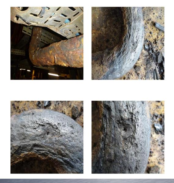
Defects on high pressure pipework are more likely to overpressure and burst during service.
