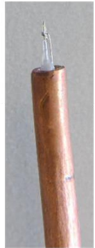
The home-made Ag/AgCl micro- reference electrode (RE), with Pt wire wrapped as CE
