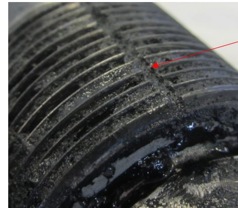
Blocked equalization ports on a solid carrier plug
