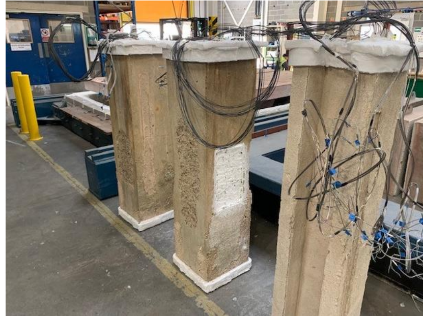
Concrete / LWC Columns post test
