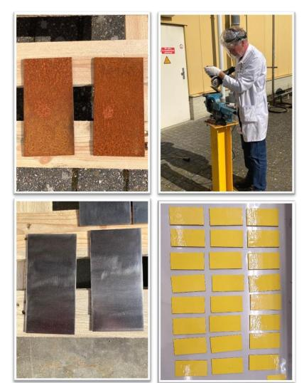
Unexposed coated panels were tested for adhesion (ISO 4624) and color (ISO 11664-4)
