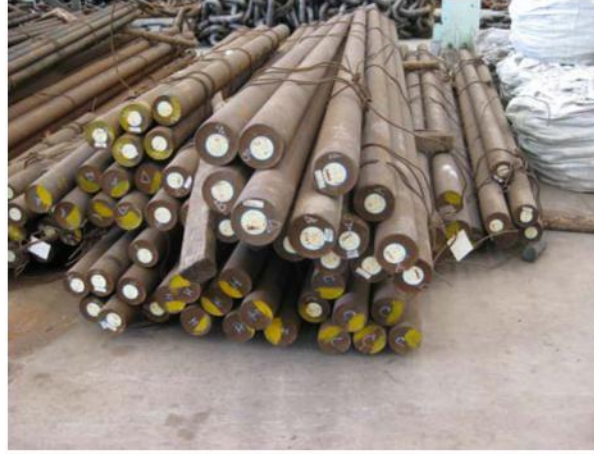
Carbon steel bars for mooring chain manufacture
