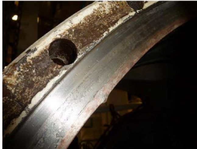
Carbon steel clad with CRA
