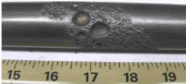
Pits on Rod Body initiated by hydrogen sulphide and brine
