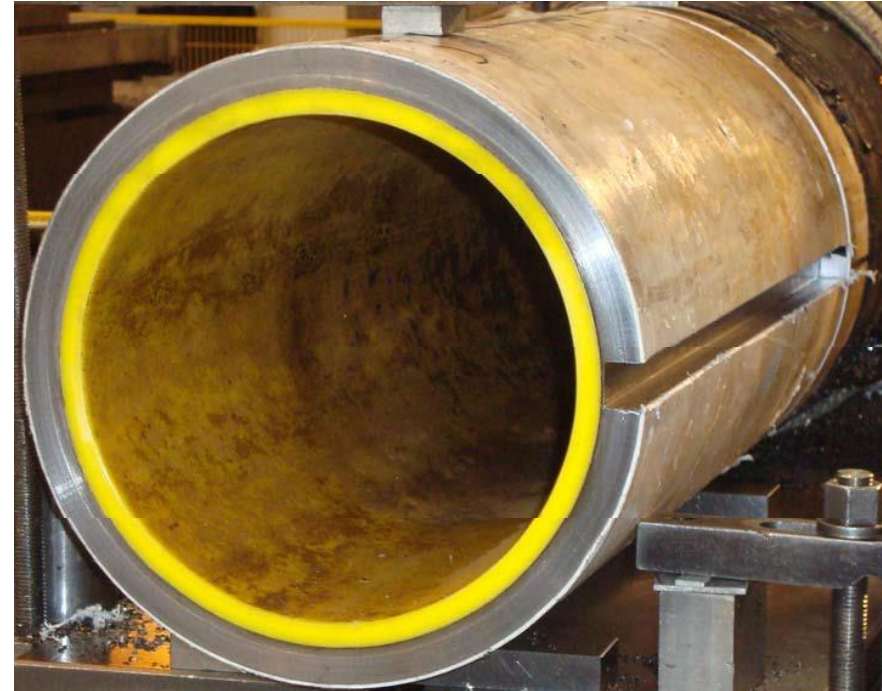
Test spool machining prior to liner pull out test
