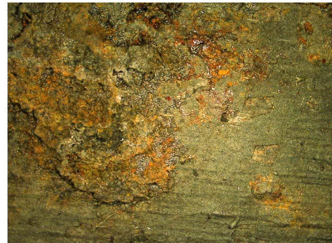
Internal surface - worst corrosion - x20 mag
