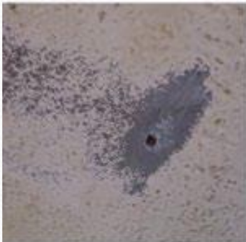
Corrosion pit: length 2x3mm, depth 1.2mm
