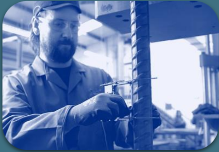
Testing of steel products for structural concrete
