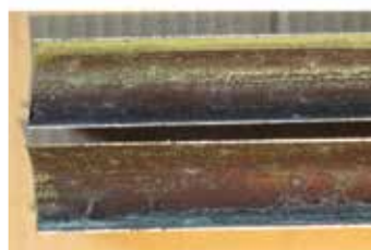
Figure 9: Pitting of CU-Ni Tubes from an MSF Desalination Plant.
