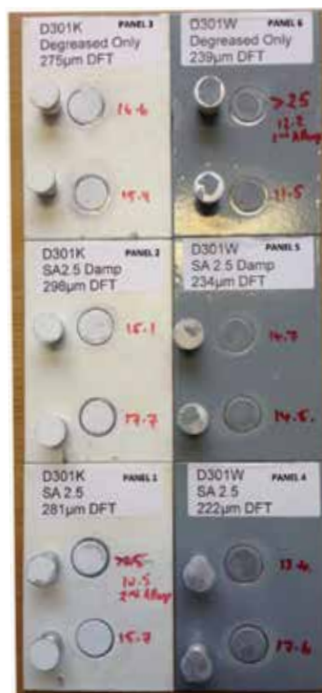
Figure 1: 301W Panels After Pull-Off Testing, Showing Failure Mode and Measured Values. Figure Also Shows Results from Adhesion Testing of A Previous Version of The 301 Series.
