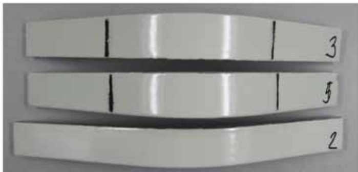
Figure 2: 301W Flexibility Samples After 4-Point Bend Testing.
