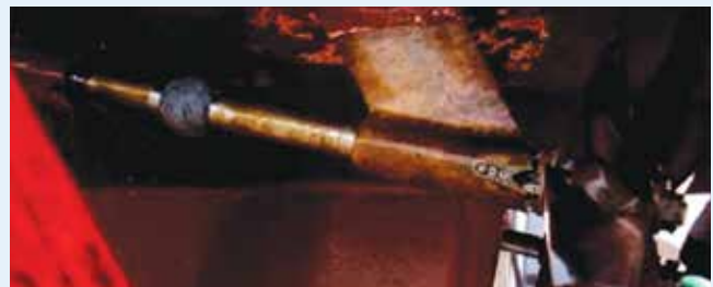
Photo: Duplex SS Propeller Shaft in-Situ with Zinc Bracelet Anode.
