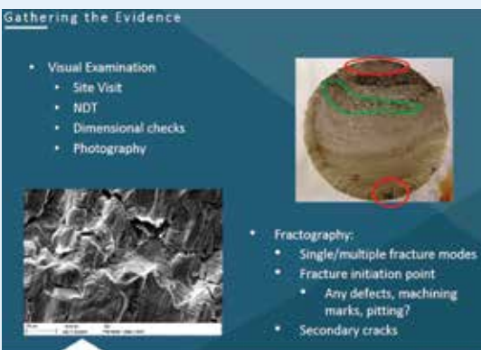
Photos: Metallographic Examination of Materials by Sectioning for Grain Structure and Crack Presence. Fracture Surface Study by Stereographic and Scanning Electron Microscopy (SEM).
