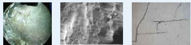
Photos: Stereographic Image of Fracture, SEM Image for Surface with XRF Analysis and a Metallographic Section Showing Crack Character.
