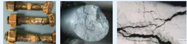
Photos: 304 SS Bolts, Cleaned Fracture Profiles, with Metallographic Section of Cracking and Grain Boundary Structure.
