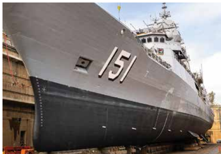
Figure 3: HMAS Arunta - an Anzac-Class Frigate of the Royal Australian Navy (RAN) Showing Zinc Galvanic (Sacrificial) Anodes Along the Hull.
