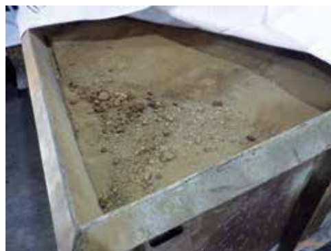
Photo 2: Ash Also Known as Zinc Ash or Skimming's from the Hot Zinc Bath. These Imperfection Can Cause Adhesive Impairments.
