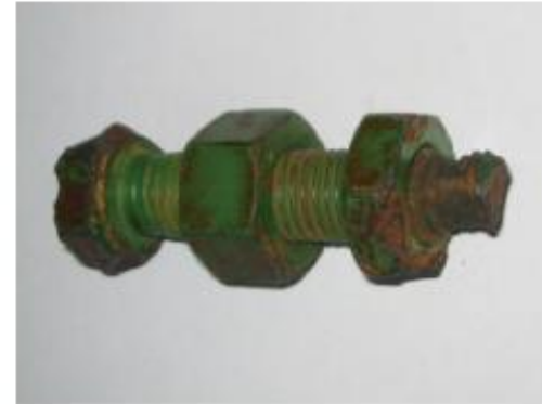
Figure 10: PTFE coated subsea fastener (source: EEMUA Publication 194)
