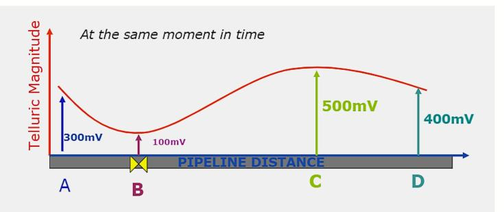
Regional Effects on pipeline structures on telluric variation: Valves, bends, rectifiers, anodes, insulating flanges
