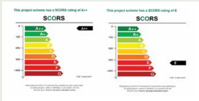
Figures 8 & 9 – SCORS Rating for GACP and Full Deck Replacement, Respectively.
