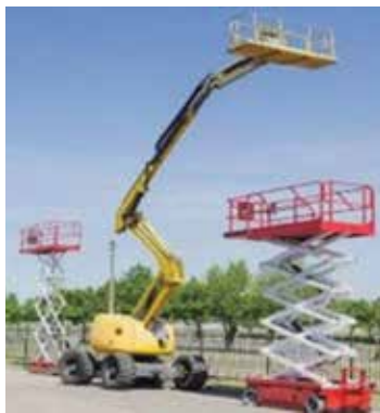
Photo: MEWP (Mobile Elevating Working Platform).
