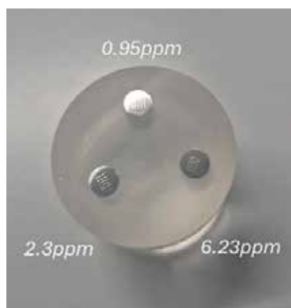
Figure 2: Mounted Hydrogen in Steel Standards with LIBS Shot Ablation Visible on Each of the Standard Surfaces.
