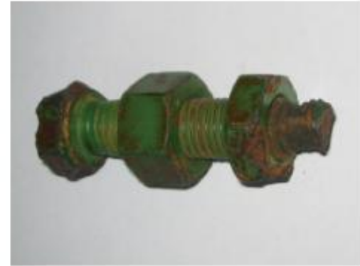
PTFE coated subsea fastener (source: EEMUA Publication 194)
