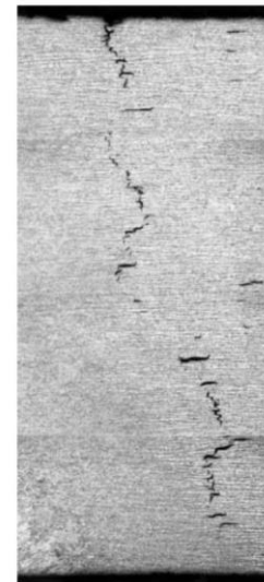
FIGURE 2—SOHC in Carbon Steel Under Applied Stress. Direction of tensile stress is normal to cracks linking the blisters.
