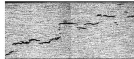
FIGURE 1—HIC in Carbon Steel Under No Applied Stress
