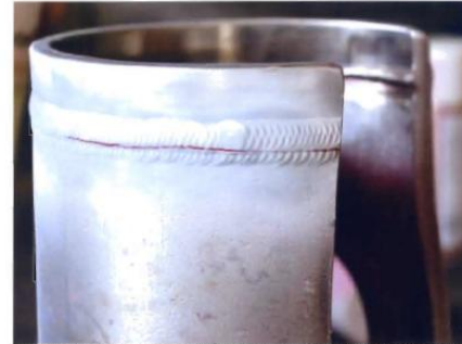
Figure 2: Crack revealed by DP-outer diameter (110 mm approx.).
