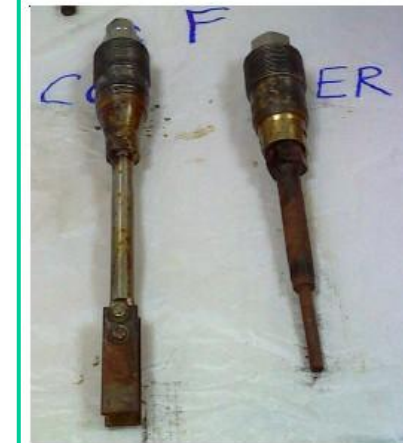
Figure 21D- CC & ER probe; location F; as retrieved condition.
