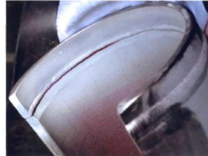
Figure 3: Crack revealed by DP-inner diameter (130 mm approx.).
