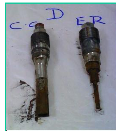
Figure 21C- CC & ER probe; location D; as retrieved condition.
