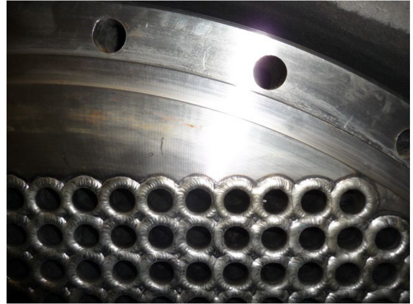
Corrosion resistant alloy (CRA) for tubes and a heat exchanger tube-sheet
