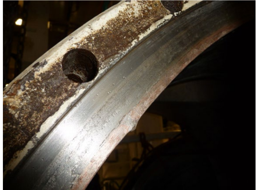
Carbon steel clad with CRA
