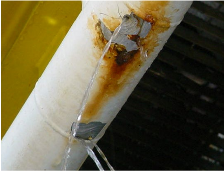
Chloride stress corrosion cracking
