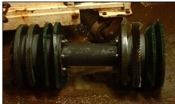
Operational cleaning pig
